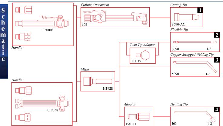
1 = Cutting 2 = Welding with Flexible Tip - Medium Pressure 3 = Welding with Single Flame - Medium Pressure
